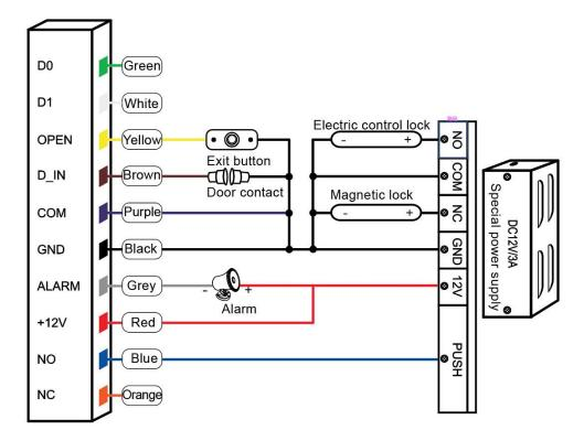
Note: The door contact and alarm function are optional
