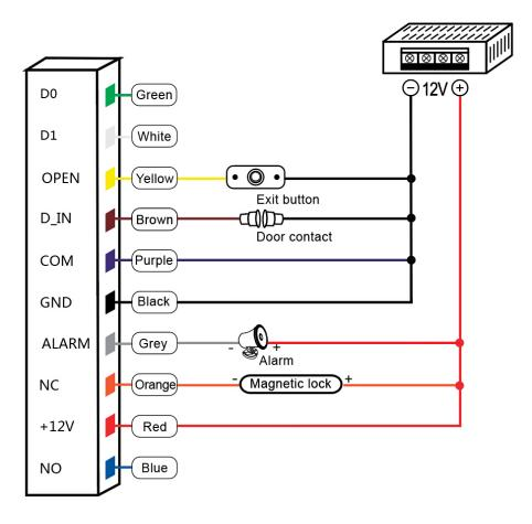
Note: The door contact and alarm function are optional
