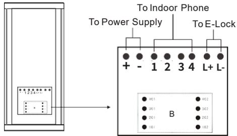
LOCK+ Connects with lock. This line can be signal line for unlocking if it is not used for the lock. Available for high level (12V)
